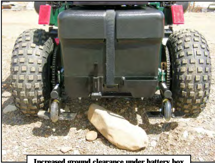
Increased ground clearance under battery box
