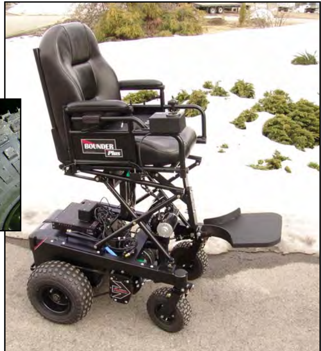
Bounder Plus H-Frame with Panther drive, PSE2 power seat elevator and 50 degree power tilt, shown in the elevated position
